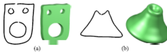
Figure 2: Sketched 2D curves can also be used to create (a) linear sweeps and (b) surfaces of revolution.
