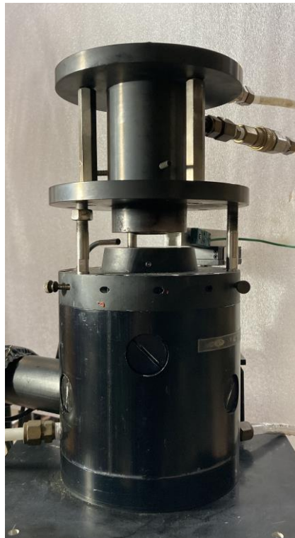
Figure 8: Counterflow burner in extinction configuration at the University of California, San Diego
