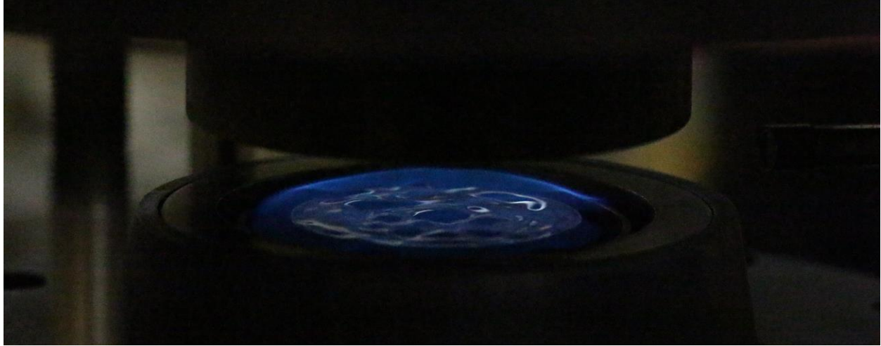
Figure 17: Bubbles on the surface of the mixture 20 vol% ethanol and 80 vol% decane during an extinction experiment with an oxygen mass fraction of 0.19
