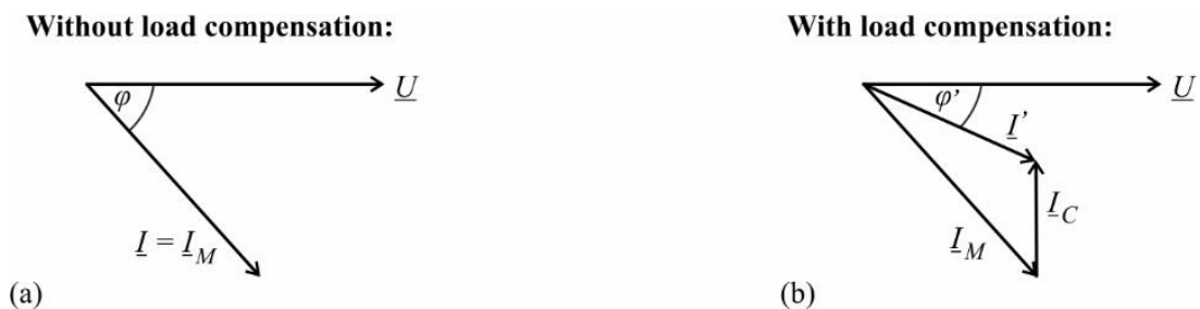
Fig. 3.10 Vector diagrams of induction motor: (a) Without load compensation; (b) With load compensation at the device level.
