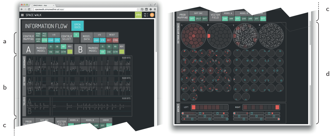
Figure 3.5: A screenshot of the Information Flow plugin. It shows a) general and model specific settings b) the visualisations of the model-action mismatch c) visualisation settings for the exploratory model visualisation d) extensive visualisation for linear and circular analogue inputs.
