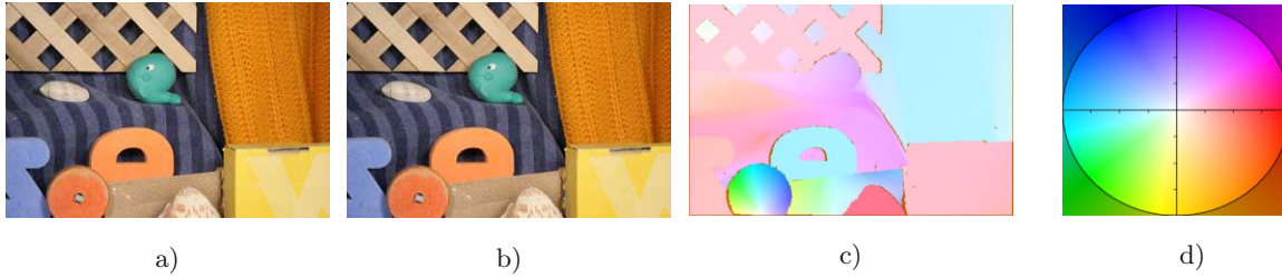
Fig. 5.2: OF visualization using color coding. The OF field corresponding to the temporally successive images depicted in a) and b) is visualized in c) using color coding. For reference, in d) we show the color pattern corresponding to a diverging OF field, with the OF magnitude increasing proportionally to the distance from the center. Note that OF orientation and OF magnitude are represented by hue and saturation, respectively.
