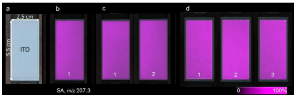
Figure S3: Testing the homogeneity of matrix coatings by the use of MALDI MSI.
