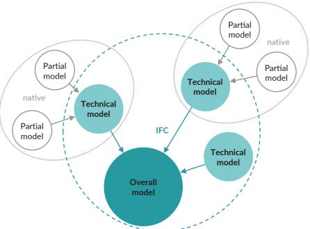
In contrast exists the system of a central model in which all specialist planners work together on a central model using one software application (software family). This is referred to as closedBIM. Mixed forms are also possible. A specialist planner can work together with his planning partners in closedBIM, but operate the overall model for coordination based on openBIM via IFC.
