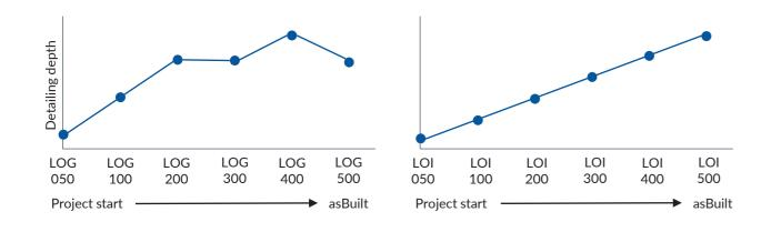
While the level of detail of the alphanumeric requirements in the LOI increases steadily, the level of detail of the LOG may be partially constant (e.g., between LOG200 for design and LOG300 for submittal planning) or even decrease at the time the asBuilt model is handed over to facility management.
