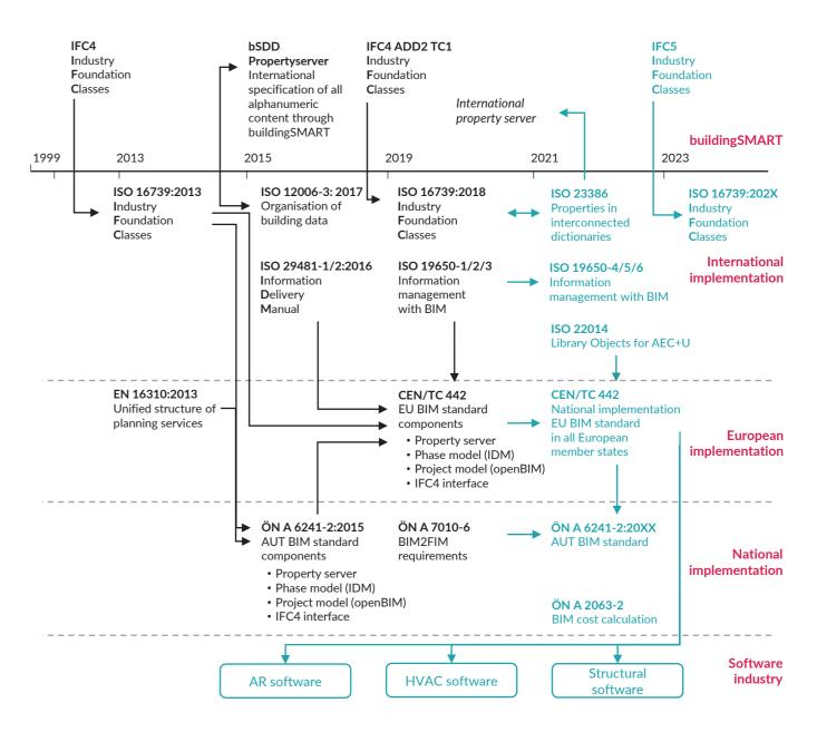
The figure above shows the dependencies of the various standards on each other in chronological order. The basis for the use of openBIM is the manufacturer-neutral data structure IFC4, which was developed by bSI and certified in 2013 as ISO standard ISO 16739:2013 »Industry Foundation Classes (IFC) for data
