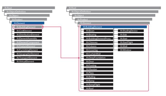
Another subclass of IfcElement is IfcDistributionElement, which contains elements for distribution systems used in the MEP. These elements can be used for heating and cooling systems, waste water systems, and electrical systems, among others.
