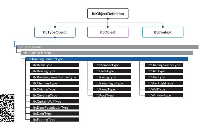
For a covering (IfcCovering), there could be the following type declarations: Ceiling, Flooring, and Insulation. Some element classes such as IfcWindow, IfcDoor and even IfcPile have multiple type declarations. The type declarations for IfcPile include, for example
