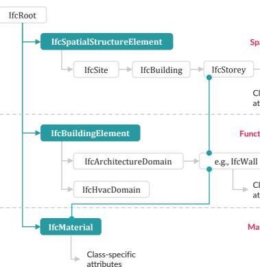
All functional elements are linked to floors and are thus also associated with a building. In addition to alphanumeric (attributes, parameters, and characteristics) and geometric information, an IFC file also contains object relationships.
