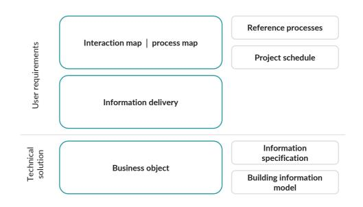
In the interaction between the individual ISO and buildingSMART standards, the IDM fulfills the task of accurately describing the defined processes for an MVD (IFC schema) using the bSDD and thus rendering them applicable.
