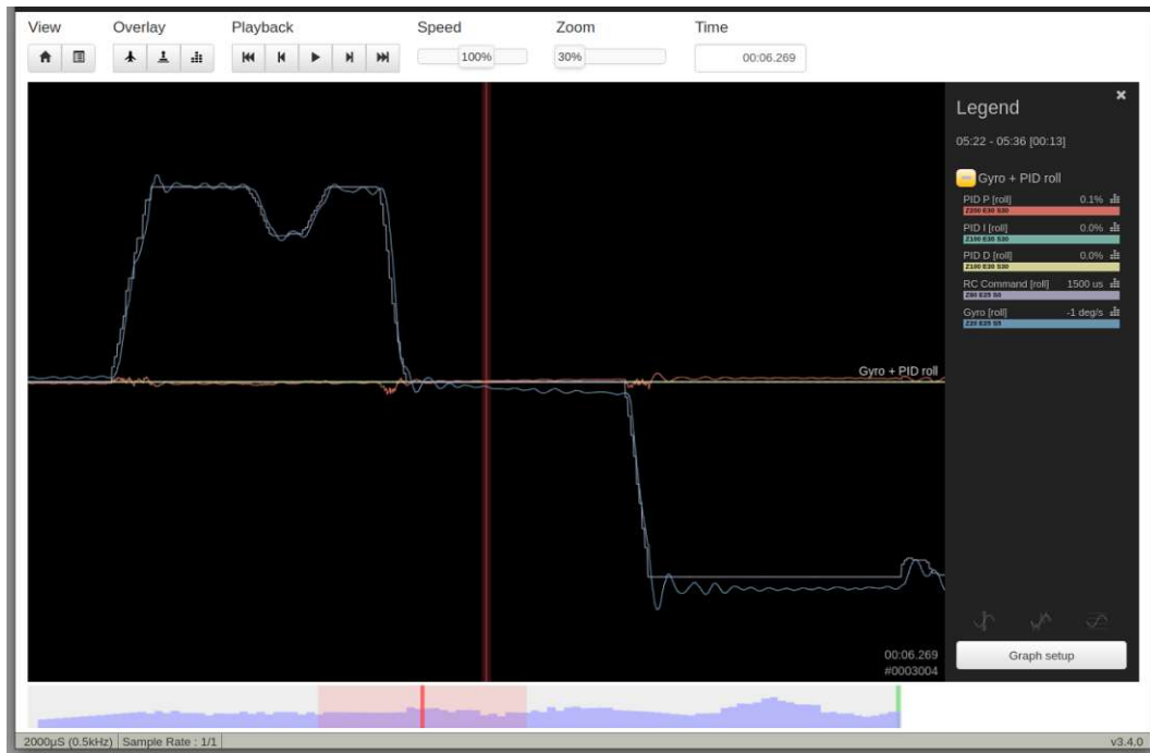
Figure 6.10: Rate Controller test for k_p = 40, k_i = 0, k_d = 0 .
