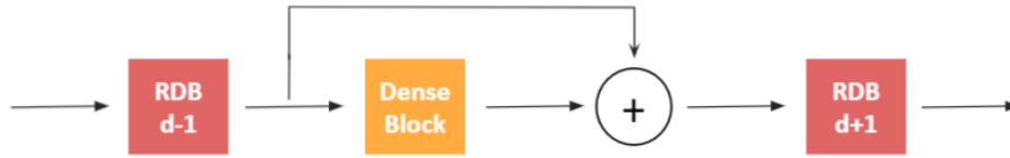
Figure 3.4: Residual Dense Block. Source: Own image based on [94]
