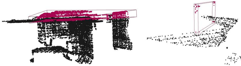
Figure 3.14: Two examples of derived bounding boxes not passing the volume selection. Points within the bounding box are highlighted in pink. The left graphic shows a chair point cloud after an mapping loss event, the right graphic one of the initial observations of a table .
