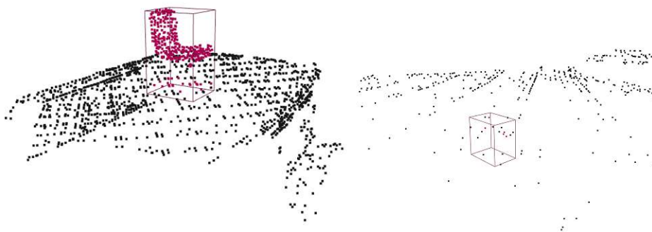
Figure 3.13: Two correctly detected objects, identified object points are colored in magenta, similar to the derived bounding box, remaining points are colored dark gray. Due to category based algorithm fine tuning correct results could be achieved also for demanding examples such as detecting the small cup the right point cloud (Image is zoomed to object points for better readability).
