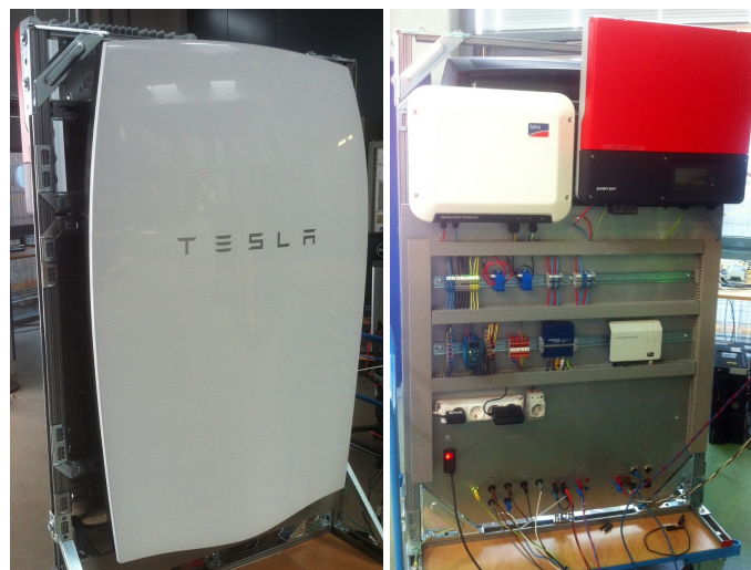
Figure 16. Laboratory setup with the Tesla Powerwall and the Sunny boy storage 2.5.
