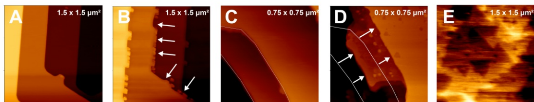
Figure 3.5: In-situ AFM topographies indicate preferential dissolution of 10\bar{1}0 step edge surfaces on a (0001) surface (marked by arrows) upon decrease of the pH values from (A/B) pH 8 to 6, and (C/D) pH 8 to pH 3. (E) shows an ex-situ topography after immersion into a pH 3 solution, indicating stabilization by formation of triangles with step edges of (10\bar{1}0) orientation on (0001) surfaces (c.f. text for details).
