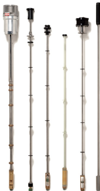
Figure 4.10: Different kinds of PPMS utility inserts [60].
