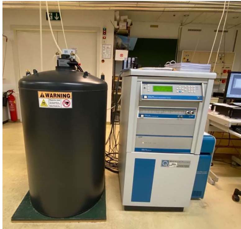
Figure 4.11: PPMS consisting of a cryostat (black dewar left) and a controller (right).
