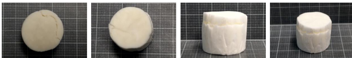
Figure 16: Samples destroyed during freeze drying, showing large cracks
