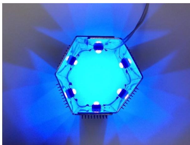
Figure 15: Lamp array with a wavelength of 400 nm working under 0.20 A and 18.9 V. The sample should be placed in the centre of the lamp to get best photopolymerization results.
