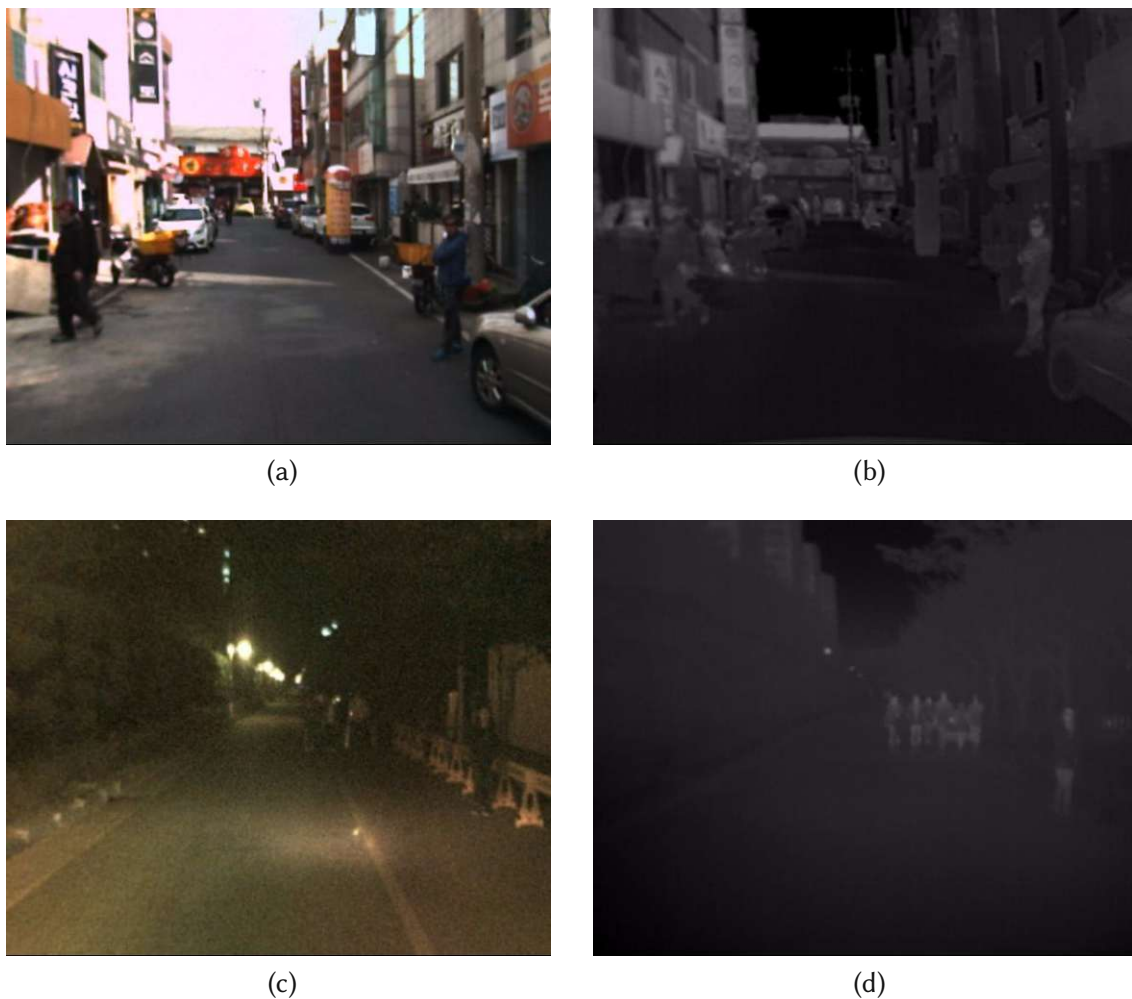
Figure 3.1: Example image pairs of the KAIST dataset: (a) Day scene RGB image; (b) Day scene LWIR image; (c) Night scene RGB image; (d) Night scene LWIR image.
