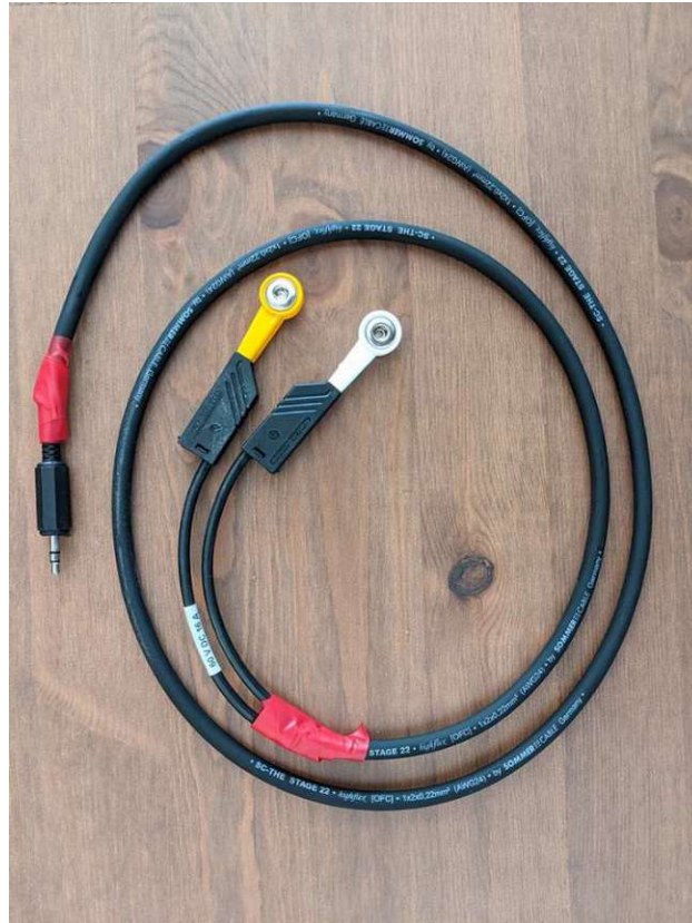
Figure 5-10- The final electrode design using a shielded microphone cable, a 3.5mm phone connector and two banana plugs ending in a connecting plug for the electrode pads
