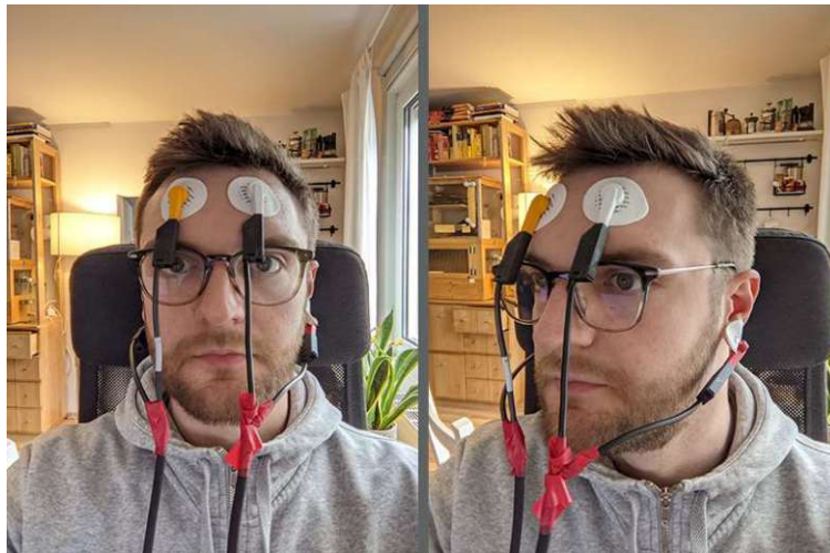
Figure 6-2 Electrode placement according to the 10- 20 system. Fp1 and Fp2 are used and A1 and A2 are the corresponding reference points.
