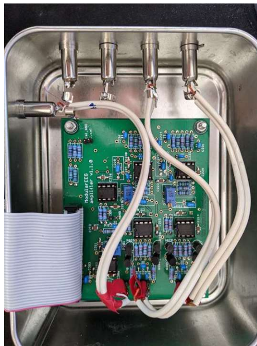
Figure 5-6 – The analogue board inside the casing. The female 3.5mm phone jacks can be seen at the top and the left of the image. Note that the two left inputs are not connected in the top row as they are a leftover from a previous design.
