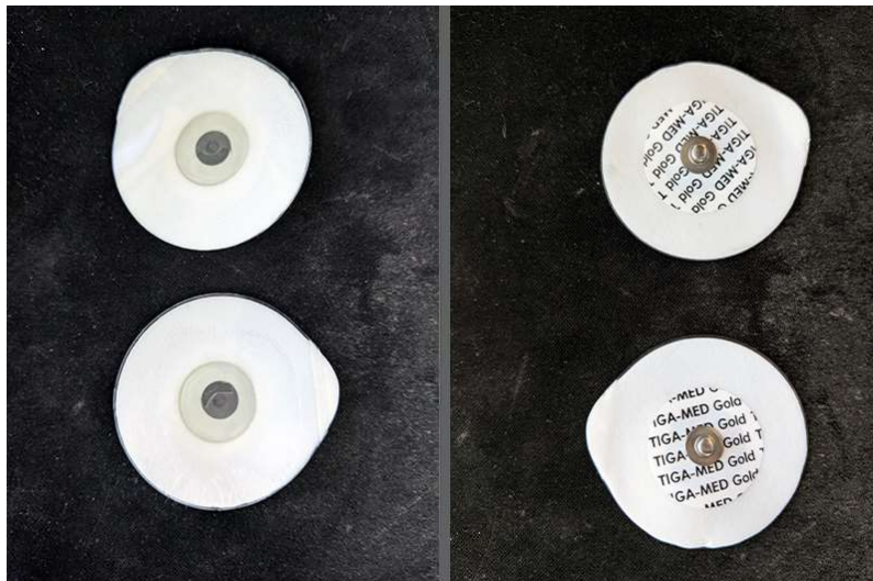
Figure 5-9 – Left: Silver-chloride patch of the electrodes visible in the center. Right: Connecting pin for measurements on the back of the electrodes
