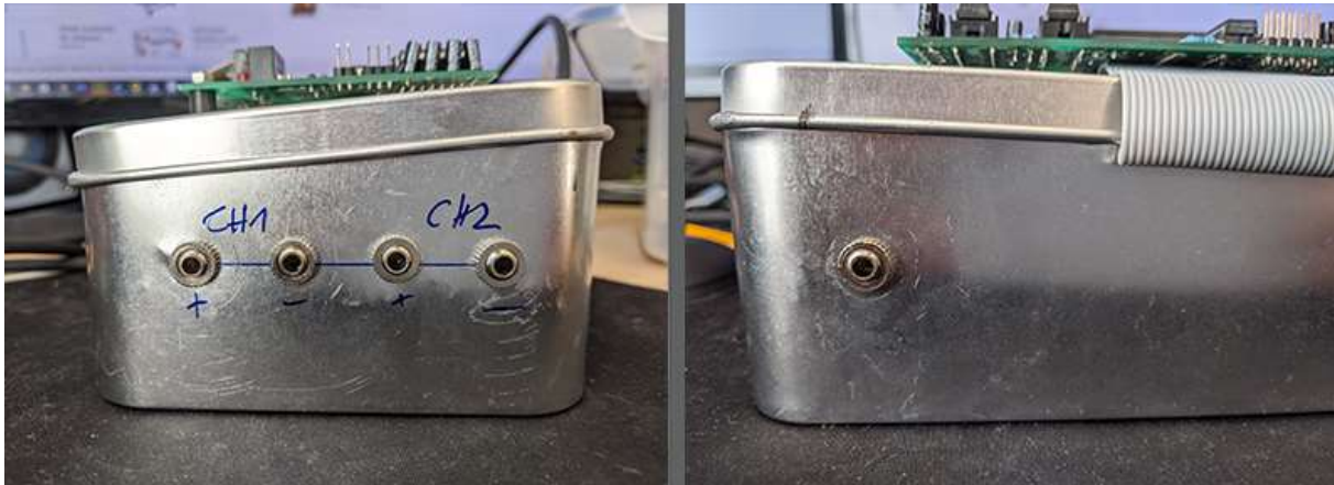
Figure 5-7 – Left: Input connectors for electrodes. The existence of 4 plugs is a relict of an earlier design trial. Only the two ports marked as CH1 are active and each of them is used to plug in one channel. Right: Input for the DRL electrode.
