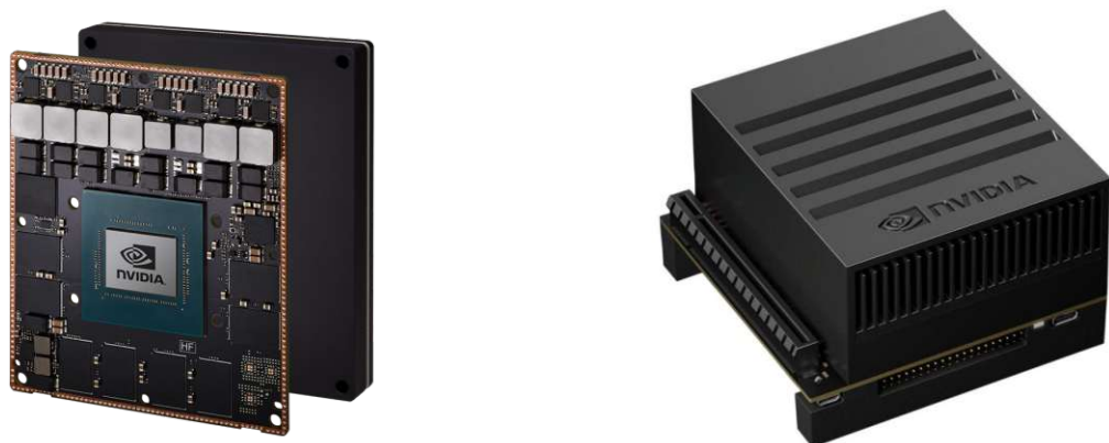
(a) NVIDIA Jetson Xavier AGX standalone module (b) NVIDIA Jetson Xavier AGX Developer Kit
