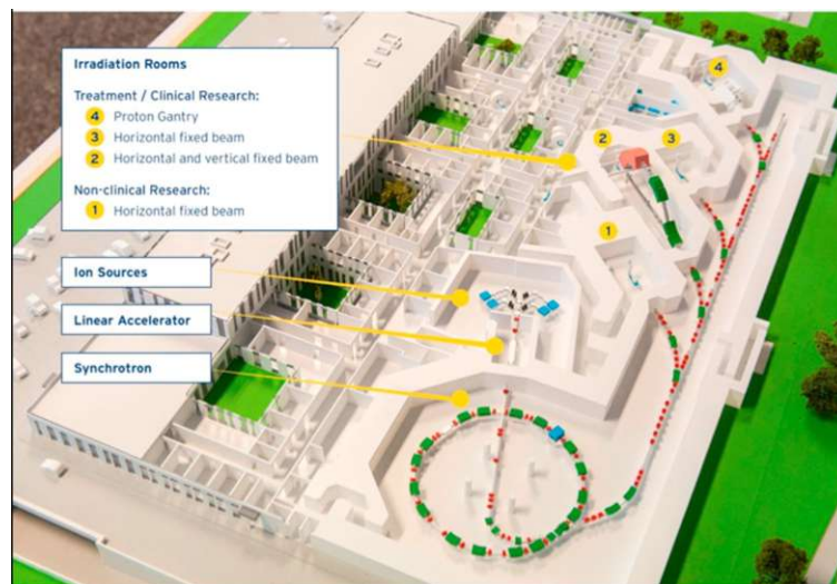
Abbildung 3.1.1: Schematic of the MedAustron facility. IR1 is for non-clinical research. IR2, IR3 und IR4 are for patient treatment either with protons or carbon ions [50].
