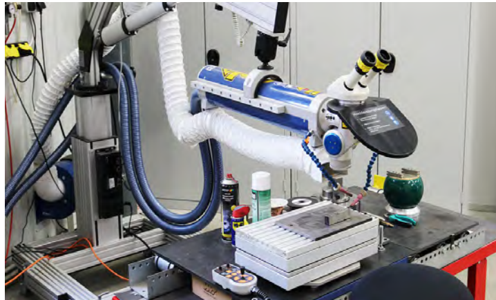
Figure 4.5: The 500 W Nd:YAG laser welding machine with adjustable head and other equipment. Source: [5]
