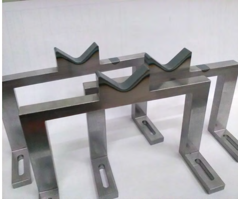
Figure 3.61: The grippers were made to pick up shaft-like parts from a pallet. Source: [5]
