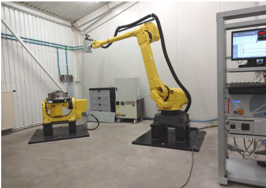
Figure 4.4: The Fanuc robot with zoom optics on the end of the arm. In the black conduit contains the pressed air for the crossjet, the cooling water for the head and the glass fiber. Source: [5]
