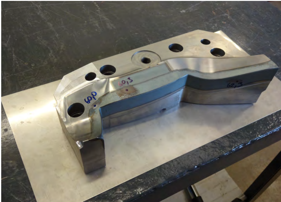
Figure 3.41: Deep drawing tool, automotive industry. Source: [5]
