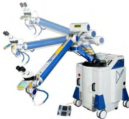
Figure 2.2: Alphalaser ALM for laser welding. Source: [6]
