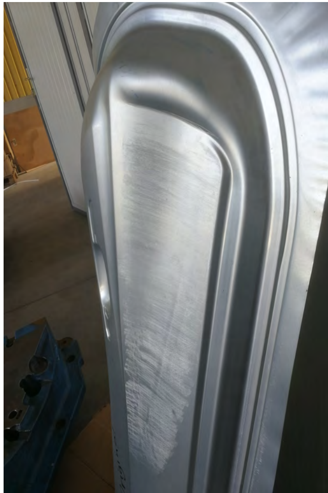
Figure 3.22: Scratches on the drawn car part due to the bad tool surface - scratches appeared on the tool because of the low hardness. Source: [5]
