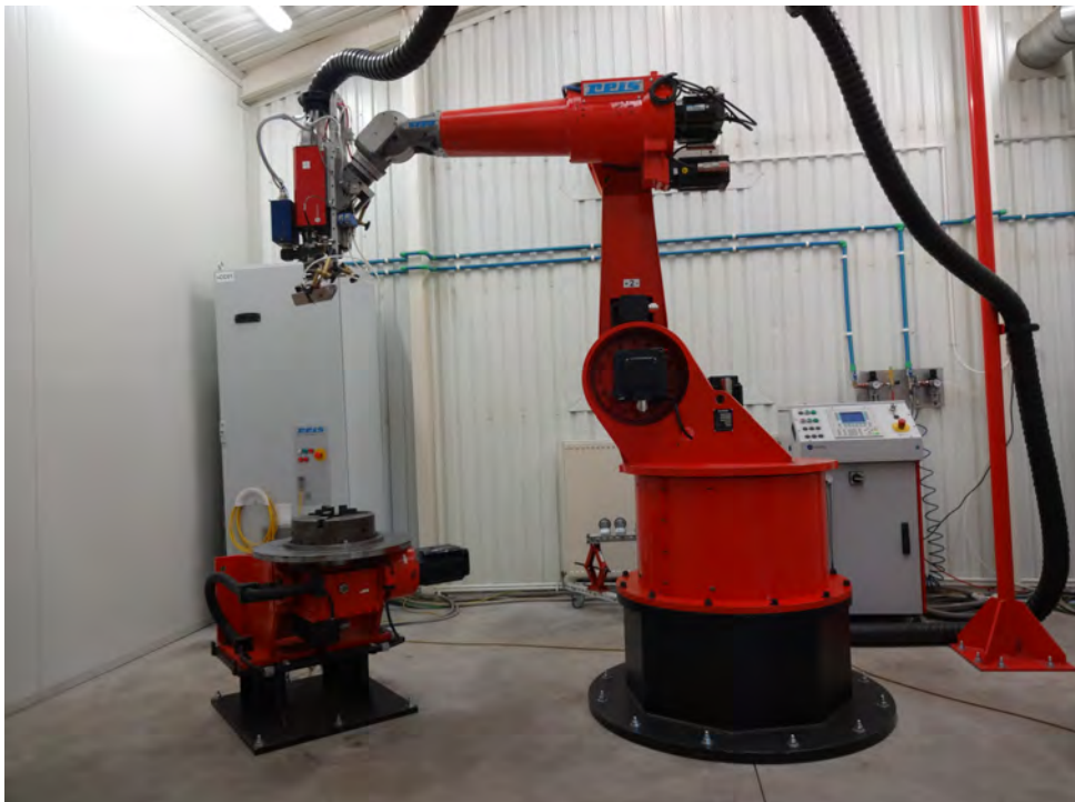
Figure 4.3: The Reis robot with the 3 kW diode laser mounted on the EOA. Source: [5]
