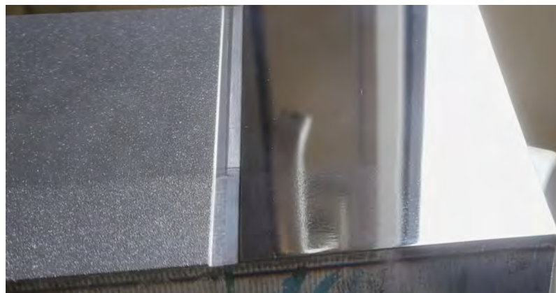
Figure 2.20: There was one laser hardened track on the surface. After polishing there's still a small difference between the original and the hardened. Source: [5]
