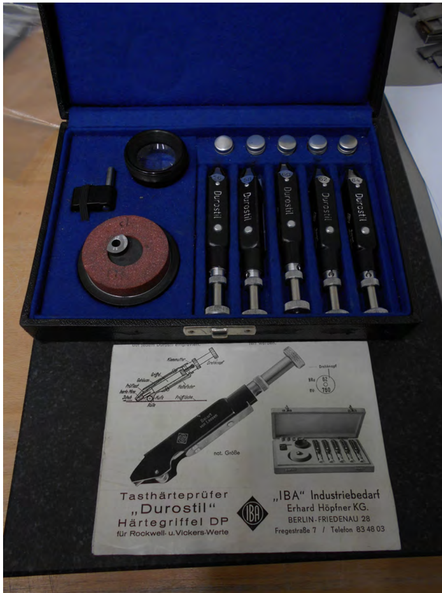
Figure 3.6: Scratching hardness testing set from IBA. Source: [5]
