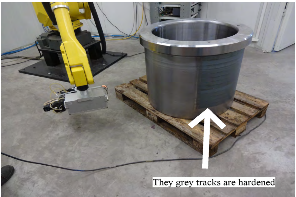
Figure 3.59: Huge piston for hydraulic pressing machine. Source: [5]
