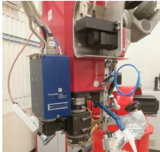
Figure 3.12: The camera is mounted on the optics on the EOAT (End Of Arm Tool). The blue box is the thermographic camera module. Source [5]
