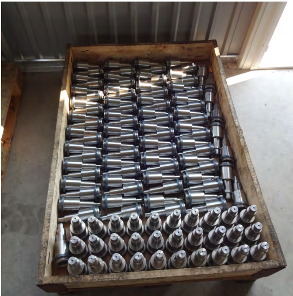
Figure 2.25: Smaller series made of C45 (1.1730) after laser hardening ready for shipping. Only the biggest diameter was hardened, around the circumference. Source: [5]
