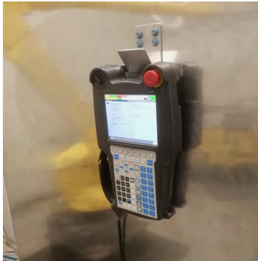
Figure 3.16: Teach pendant with the safety button. Source: [5]
