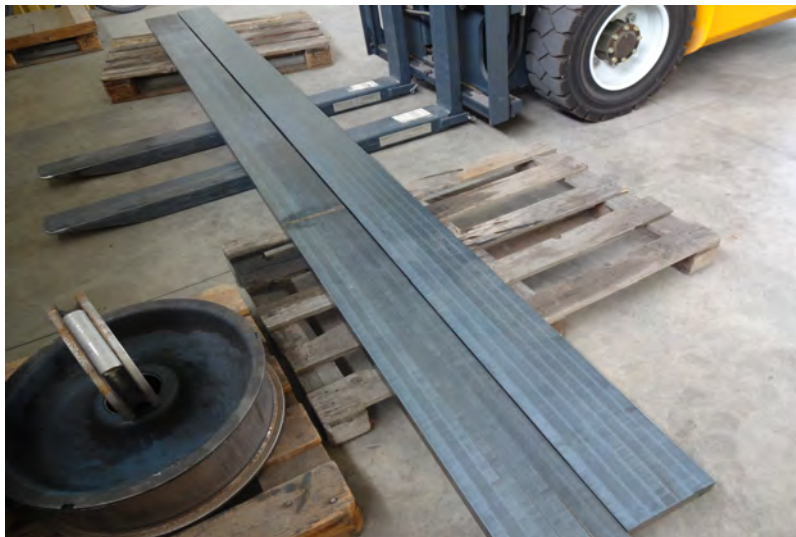
Figure 3.19: 40 mm thick guiding element, 4000 mm long after laser hardening. The material is c45, it had to be hardened both sides to equal the deformation. As a result the deformation could be pushed down under 0,1 mm/m. Source: [5]
