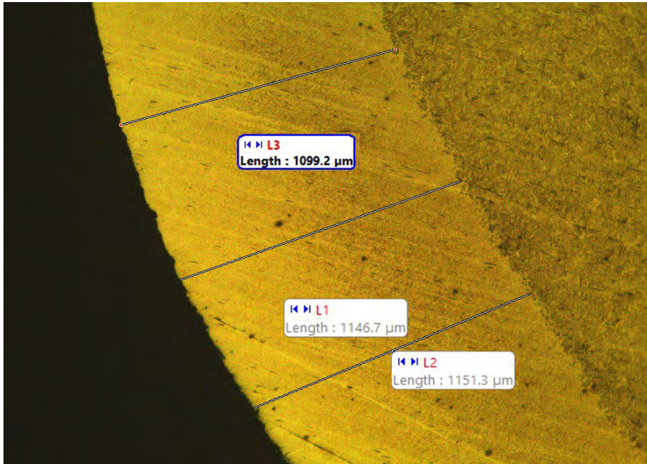
Figure 3.39: Specimen made from 1.2312, v=5 mm/s R5 mm radius etched with Nital 2%. Source: [5]
