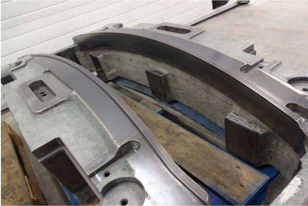
Figure 3.23: Blank holder after laser heat treatment. Source: [5]
