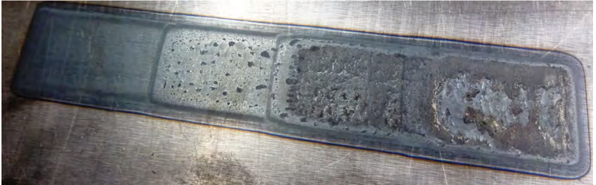
Figure 2.19: C45 hardened with different temperatures. From left to right: 1150, 1200, 1250, 1300°C. Source: [5]
