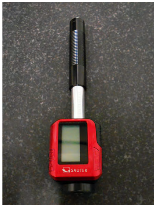
Figure 3.4: Portable Leeb tester from Sauter, Source: [5]
