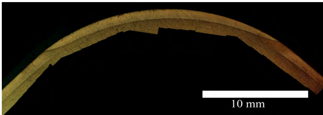
Figure 3.35: Specimen made from 1.1730, v=10 mm/s R15 mm radius etched with Nital 2%. Source [5]
