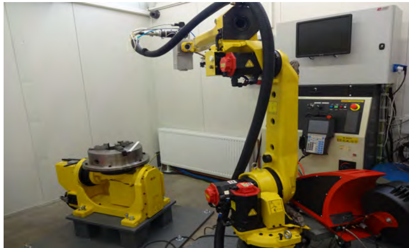
Figure 4.6: This machine is located in a smaller chamber, so it's used mainly for the hardening of smaller parts. The wire feeder is mounted on the right side of the robot (red box). Source: [5]
