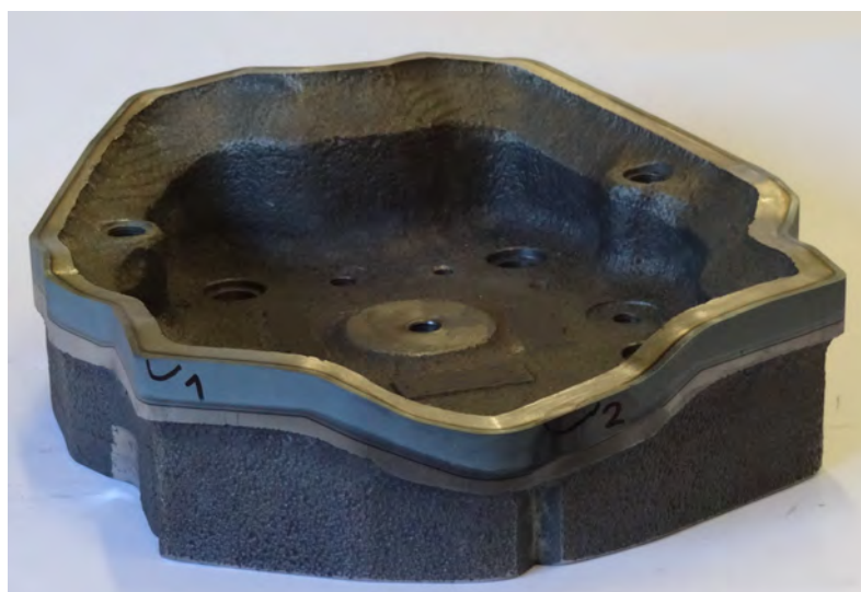
Figure 3.55: Laser hardened cutting tool from the automotive, the irradiation angle is 90^\circ . Source: [5]
