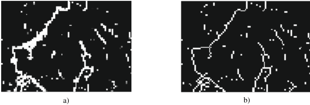
Figure 6.8: Skeletonization of a simulated crack pattern: a) original result, b) skeletonized result.
