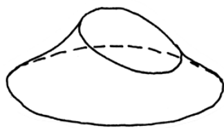
Figure 33: SDA shape CO 14 “Raked Anticlastic Cone” with modified unit shape “cone:circular:anticlastic:raked”
