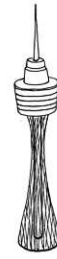
Figure 32: SDA building V 02 “Centrepoint Tower Sydney” with aggregate building shape “Cylinder:vert*2/seq:vert cone trunc top”
