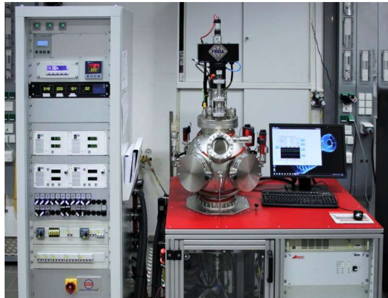
Fig. 20 Lab-scale PVD system capable of depositing carbides by reactive magnetron sputtering with acetylene (C 2 H 2 ) gas.
