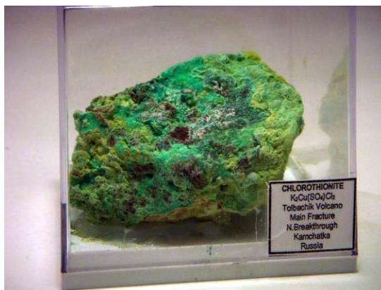
Figure 5.2: A piece of chlorothionite of roughly 8 cm, found at the Tolbachik Volcano, Kamchatka Oblast, Russia. Image taken from www.mineralienatlas.de with permission of the copyright holder Luigi Chiappino.
