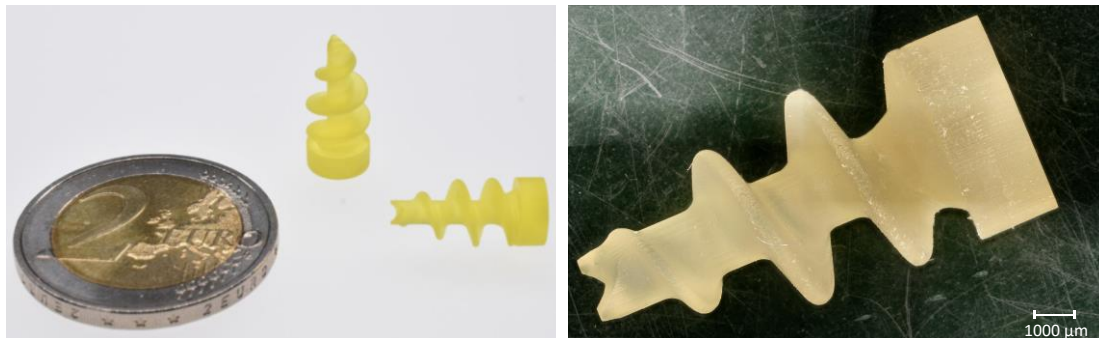
Figure 38: Microscopic image (right) of surgical screws of the formulation containing DVA, 15 db% Thiol 2 , 25 wt% AC45kPCL , 0.75 wt% Ivocerin, 0.02 wt% PYR and 0.06 wt% QY printed by digital light processing.
