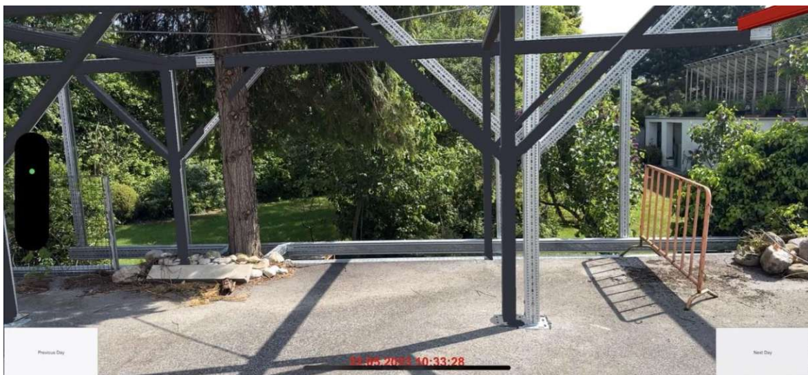
Figure 141: Possible error, when moving further away from the marker. Big inaccuracies, like depicted in this picture, only appear when the device is simultaneously screen-recording
