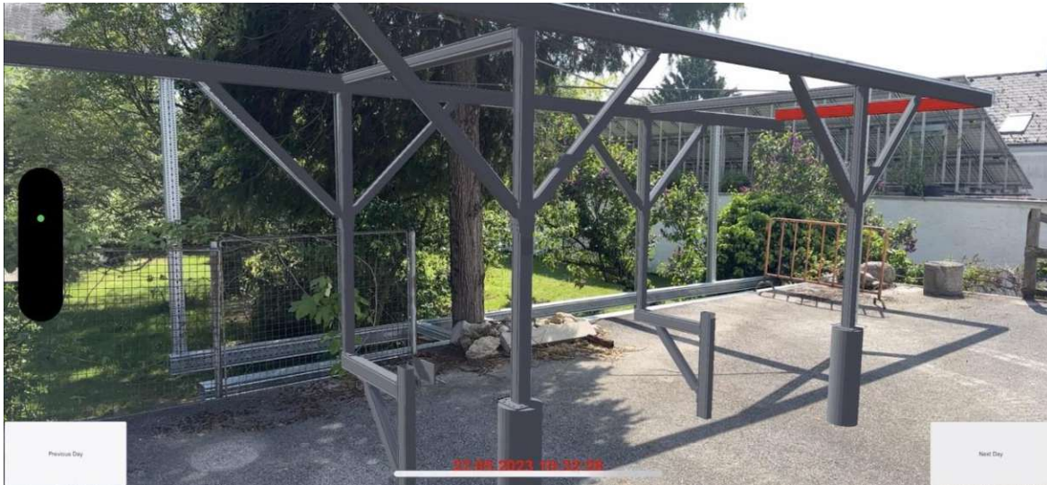
Figure 125: Augmentation without occlusion. Parts which should be behind other objects are rendered on top of them.
