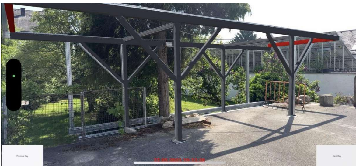
Figure 126: Augmentation with occlusion. Elements are hidden behind the 3d-modeled terrain with “Depth Mask Shader”.
