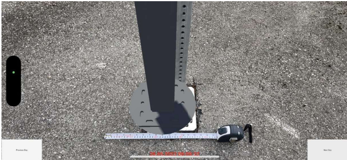
Figure 140: Detailed view of the inaccuracy of the column "Stütze-001" in axis 3. The extent is about 5cm during augmentation
