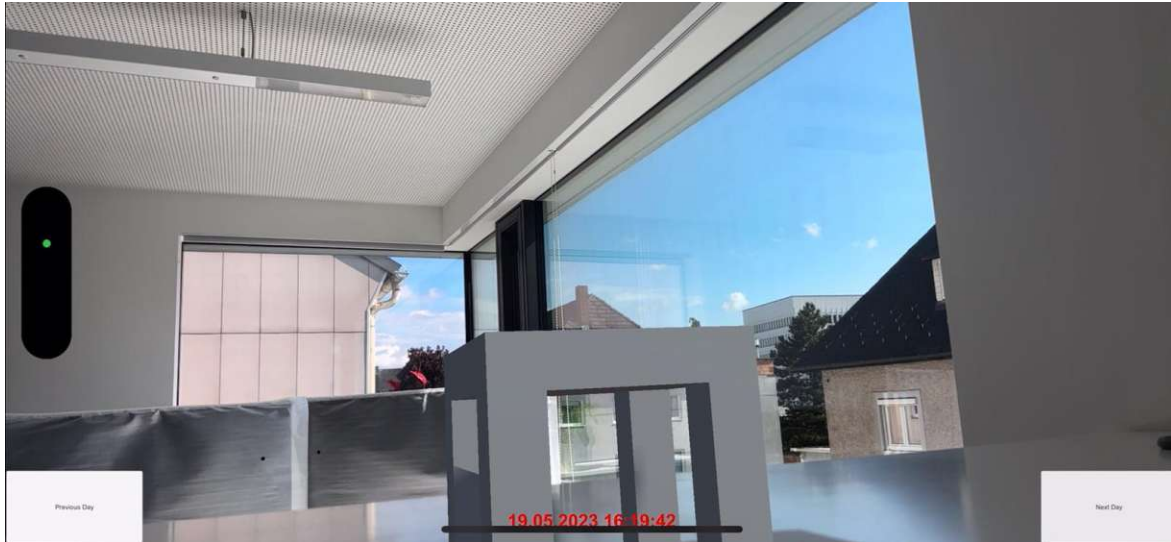
Figure 84: Test1 - when the marker is not visible in the video stream, the model still is stable and working as intended
