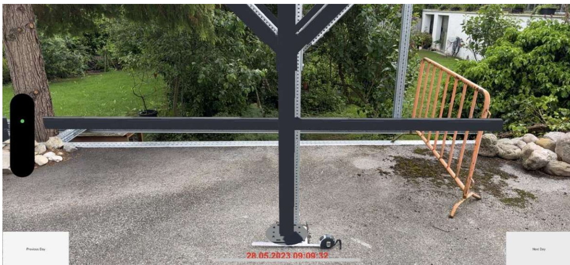
Figure 139: Inaccuracy of the structure in axis 3 when moving away from the marker. The extent is about 5cm during augmentation
