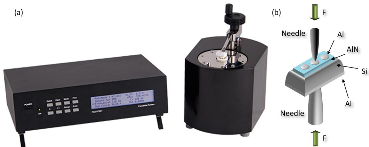
Fig. 2.15: The image shows the piezometer PM300 with an exemplary sample clamping.
