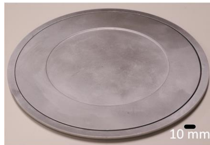
Fig. 2.6: Photo of a standard molybdenum (Mo) sample holder as provided by VonArdenne.
