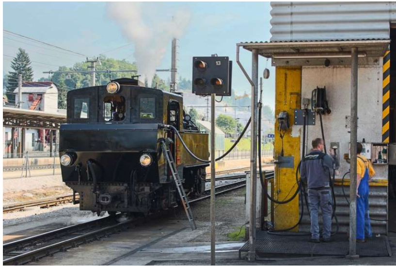
Figure 10 Locomotive No. 5 of the Zillertal Railway in the phase with oil firing while refueling at the diesel filling station (Own work , 2013)
