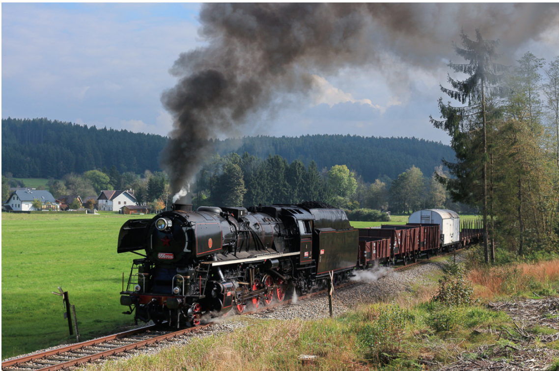
Figure 4 Czechoslovakian construction class 556: 1950s design with stoker firing at a guest operation in Austria (Own work, 2014)
