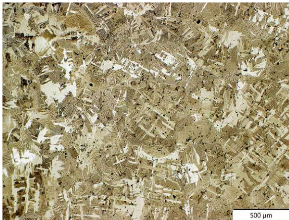
(c) Ti-6Al-4V 1000 °C/90h perpendicular
