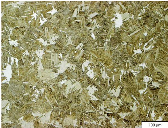
(a) Ti-6Al-4V perpendicular
