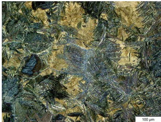
(a) Ti-6.4Ni-2Fe presintered perpendicular
