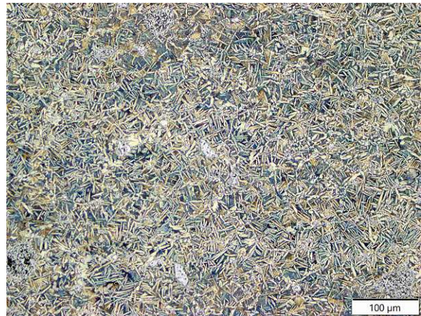
(b) Ti-6.5Cu+3vol% TiC longitudinal
