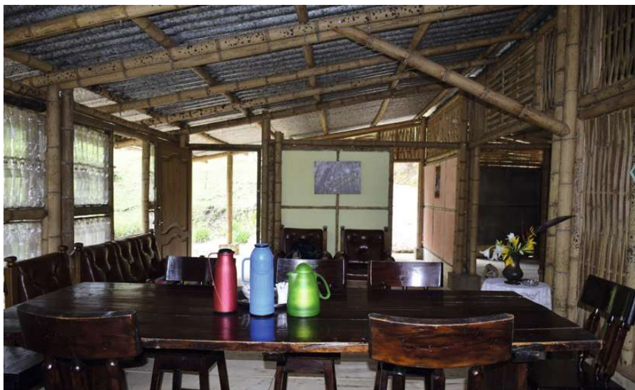
fig.85 the house is finished, with some walls left unfilled and some covered with clay.
