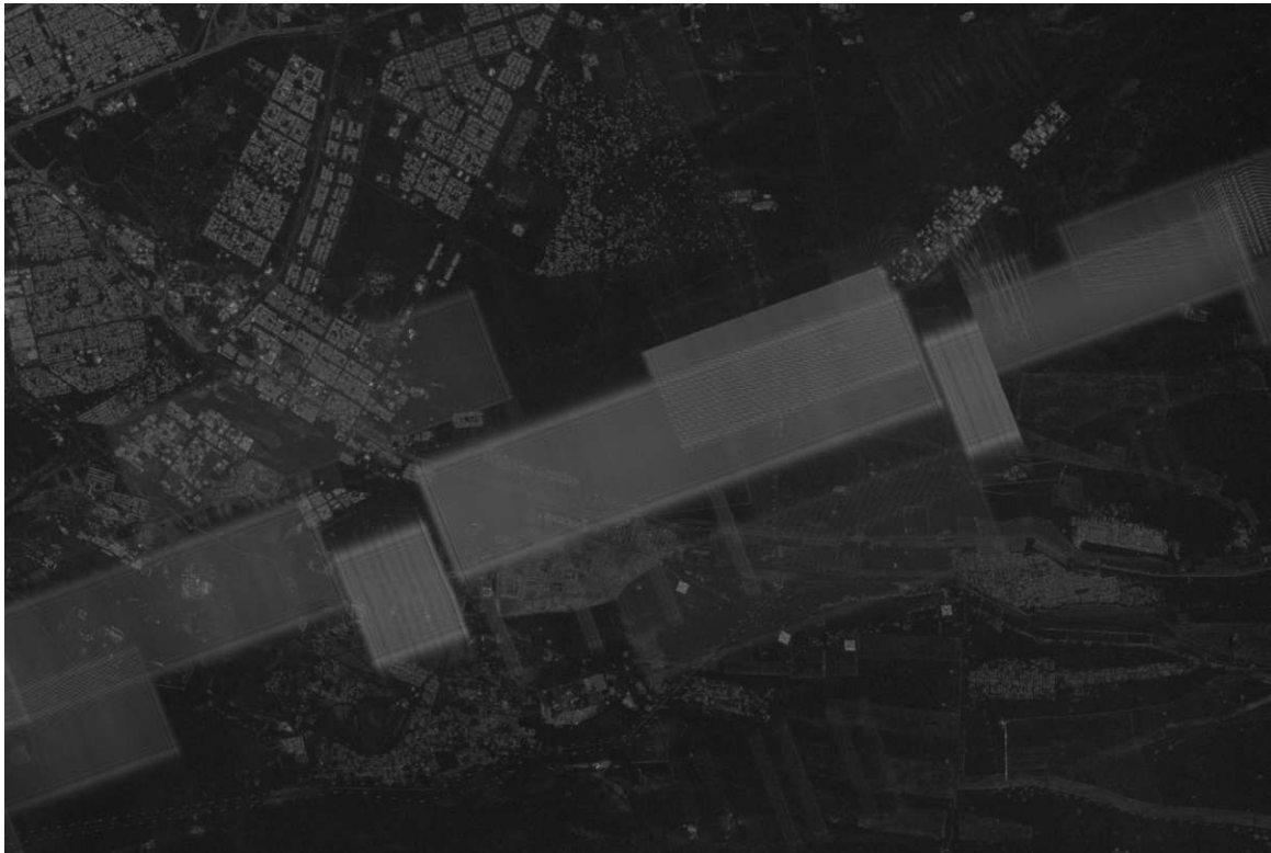
Figure 3-9. Presumable RFI effects affecting a Sentinel-1 data tile of the Abu Dhabi region
