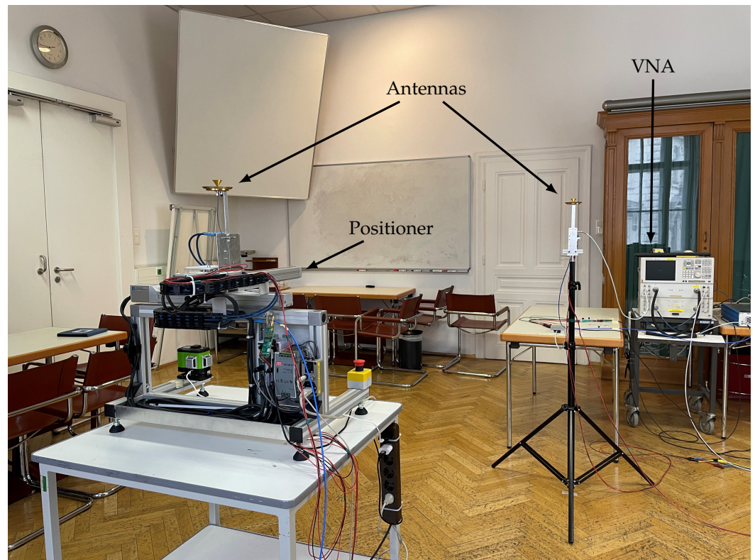
Figure 4. Channel measurement environment: seminar room at TU Wien. Specular components, e.g., walls, white board, and cabinet with glass front, as well as diffuse components, e.g., tables, chairs, and measurement equipment, are part of the interior.
