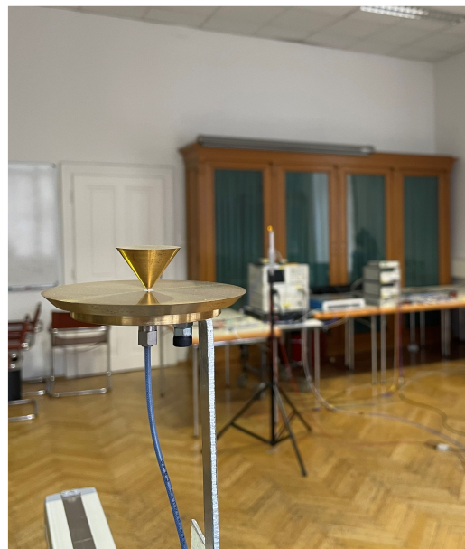
Figure 5. CMP mounted on the positioner. In the back, one of the wooden cabinets with glass fronts is seen.
