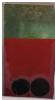
Figure 4.28: Damaged 1 wt% PDMS film on \text{Cu}_2\text{O} after the conducted LSV test.
