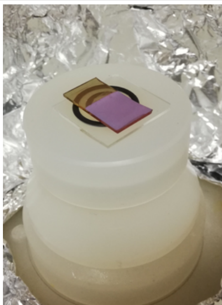
Figure 3.13: \text{Cu}_2\text{O} photo-cathode in the spin-coater machine.
