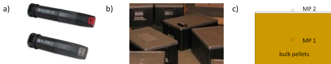
Figure 13 a) The used data loggers, b) the performance of the core temperature determination and c) scheme of the core temperature determination.
