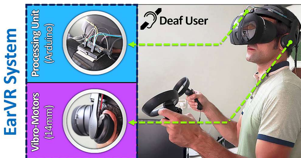
Figure 4.7: The prototype version of EarVR system designed for deaf persons.
