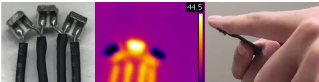
Figure 2.13: ThermalBitDisplay with three peltier device [114].
