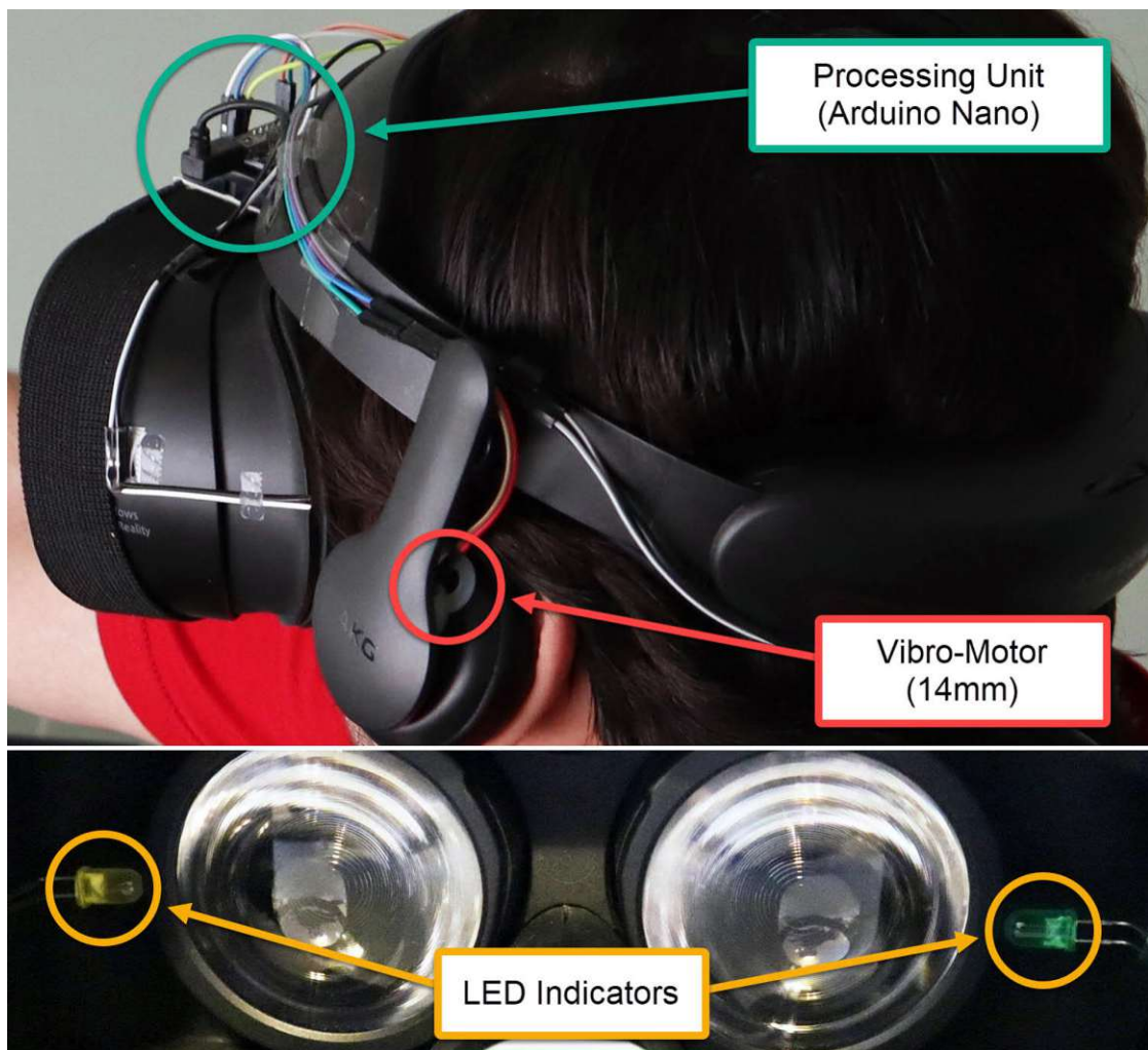
Figure 4.12: Our proposed EarVR+ system with LED indicators.
