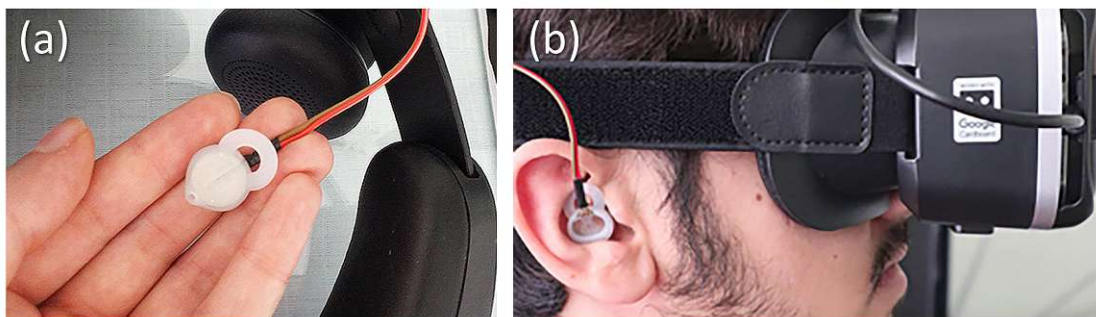
Figure 4.9: (a) Using soft cover for vibro-motors, and (b) Putting vibro-motors in the ears.
