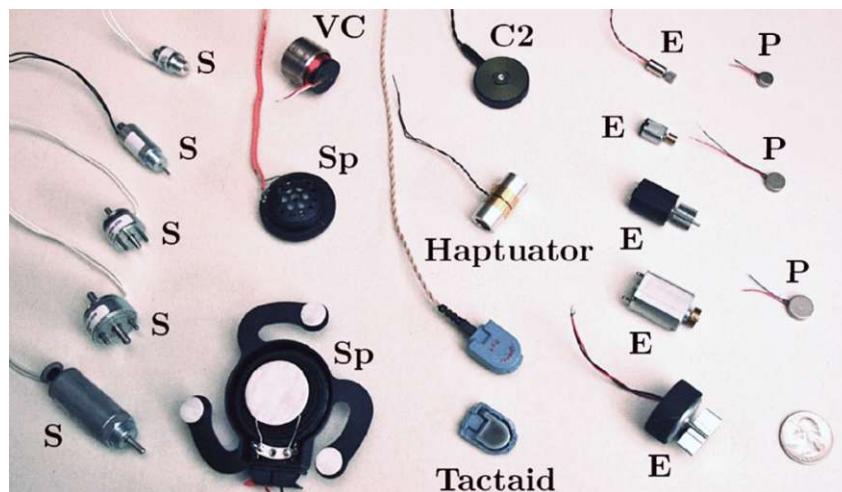
Figure 2.2: Sample actuators for vibrotactile display. *S: solenoids. *VC: Voice coil. *Sp: Audio speakers. *E: Shafted/cylindrical motors. *P: Shaftless/pancake motors. *A quarter coin for scale [77].
