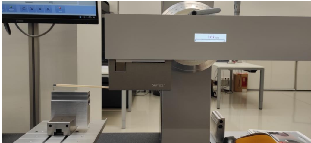
Figure 36: Surface roughness measurement process setting.
