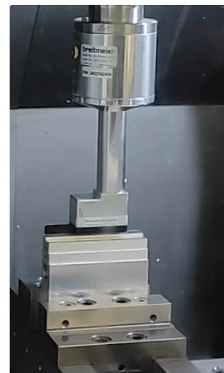
Figure 31: In-situ measurement device positioning for facemilling
