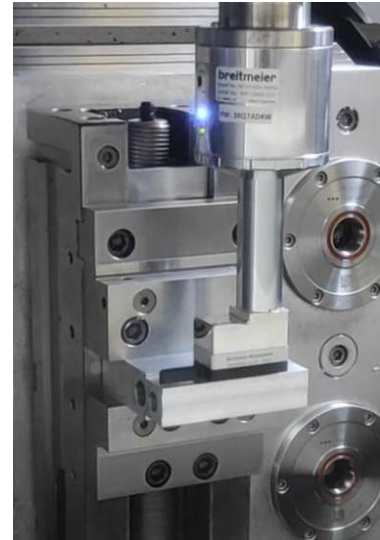
Figure 32: In-situ measurement device positioning for endmilling
