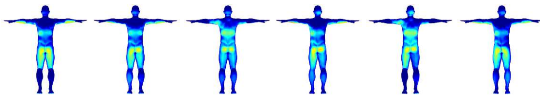
(c) Input contact pressure computed by assuming that the input body is perfectly supported.
