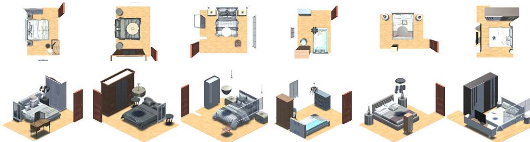
Figure 5.13: Conditional synthesis results as described in Section 5.4. All methods in a column receive the same room boundary, windows, and doors as input condition. Our approach (top row) produces on average layouts with less ergonomic issues like missing light sources (e.g. missing chandeliers in Baseline columns 1, 3 and 6) or poor accessibility (e.g. chair and wardrobe blocking the path in ATISS column 5 and 6).
