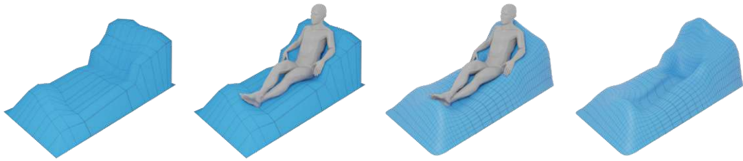
Figure 4.1: Left: seating surface generated by our automated algorithm and suited to support the input pose . Right: the surface fitting algorithm described in Chapter 3 applied to the generated surface.
