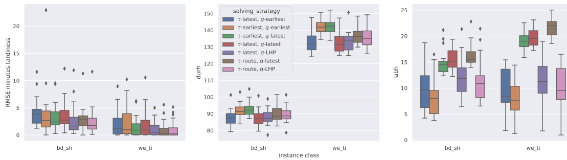
Figure 5.6: Comparison of the root mean square error of the tardiness in minutes, the travel time duration in hours, and the excess labor time in hours of different solution strategies (without offline solution) on six different instances classes with 20 instances each. We observe that the more sophisticated strategies based on LHP and the route performance decreases the tardiness at the cost of carefully introducing additional travel time (regarding which \tau -latest is best) and labor time (where q -earliest is best).
