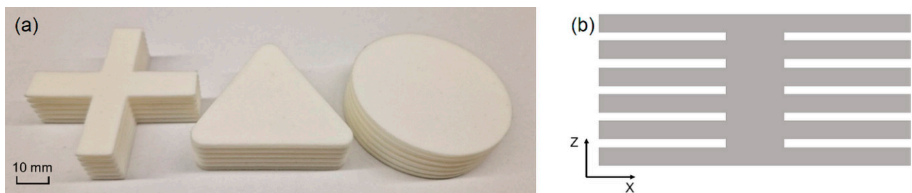
Figure 6. Different test parts in (a) as bases for further triangulation and thermal analysis: cross-, triangular-, and circular-shaped geometries and in (b) 6 identical stacked layers of 2 mm material thickness and a total height of 14 mm.
