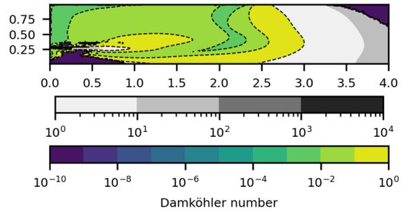
Figure 8: Damköhler number in the IFRF furnace. Values above unity are shown in greyscale.
