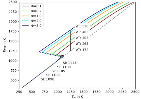
Figure 3: Ignition plot with different equivalence ratios for the Guasare coal
