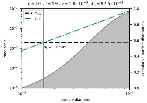
Figure 6: Additional MILD criterion from [7]. The grey area shows the cumulative particle distribution. The criterion is fulfilled for diameters larger than  $16\mu m$ .
