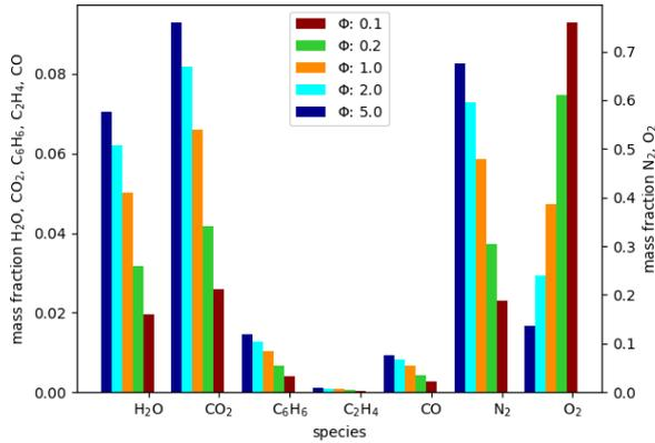
Figure 2: Different concentrations computed by the pkp-tool for the Guasare coal with varying equivalence ratios.
