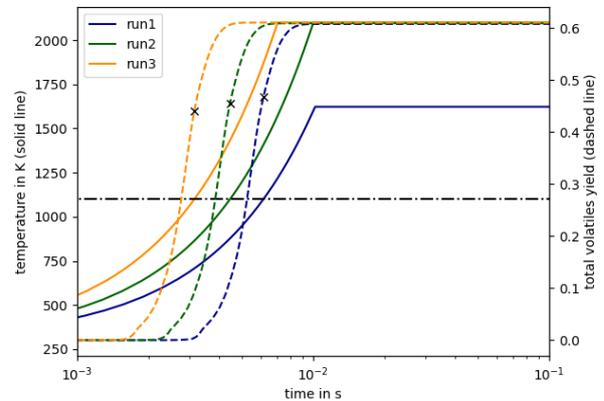
Figure 4: Total volatile yield calculated with the CPD model. The cross marks the volatile yield at self-ignition temperature.
