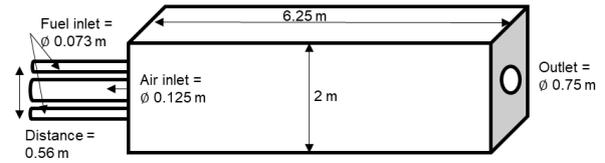
Figure 1: Schematic representation of the IFRF furnace
