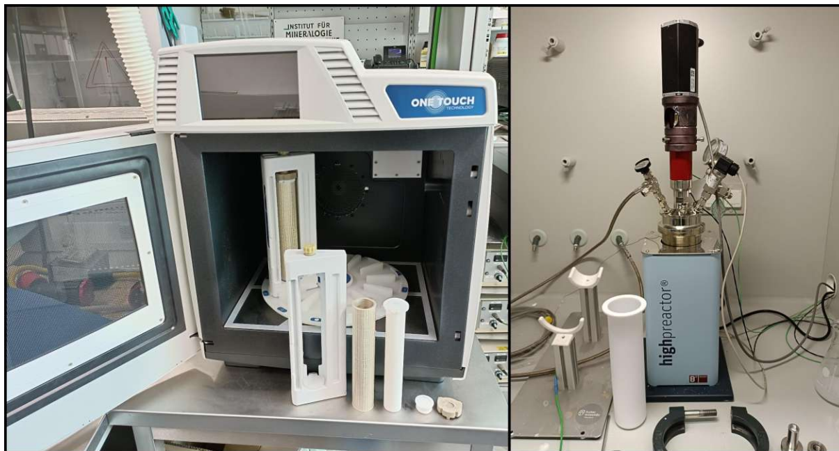
Figure 3. Left: CEM Mars6 240/50 microwave-heated furnace. Right: Berghof BW700 autoclave.
