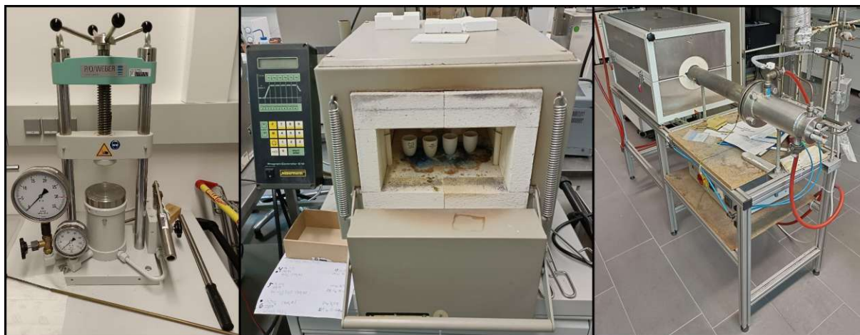
Figure 4. Left: Manual P/O/Weber PW10 press; middle: Nabertherm N11 furnace; right: FROK 500/100/1300 reduction furnace.
