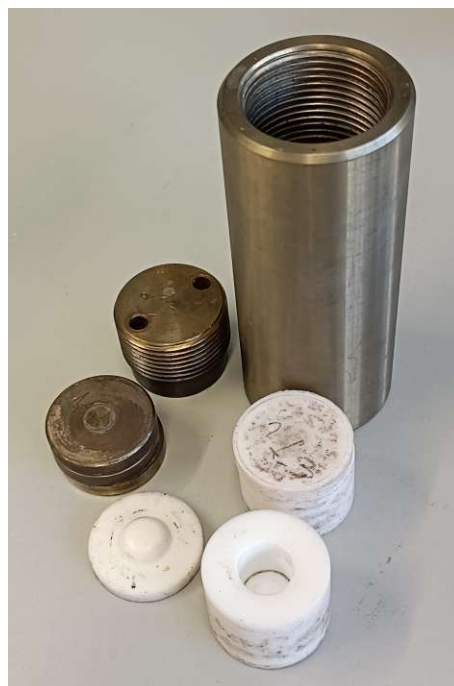
Figure 2. A set of steel autoclave and Teflon inlays used for hydrothermal experiments.
