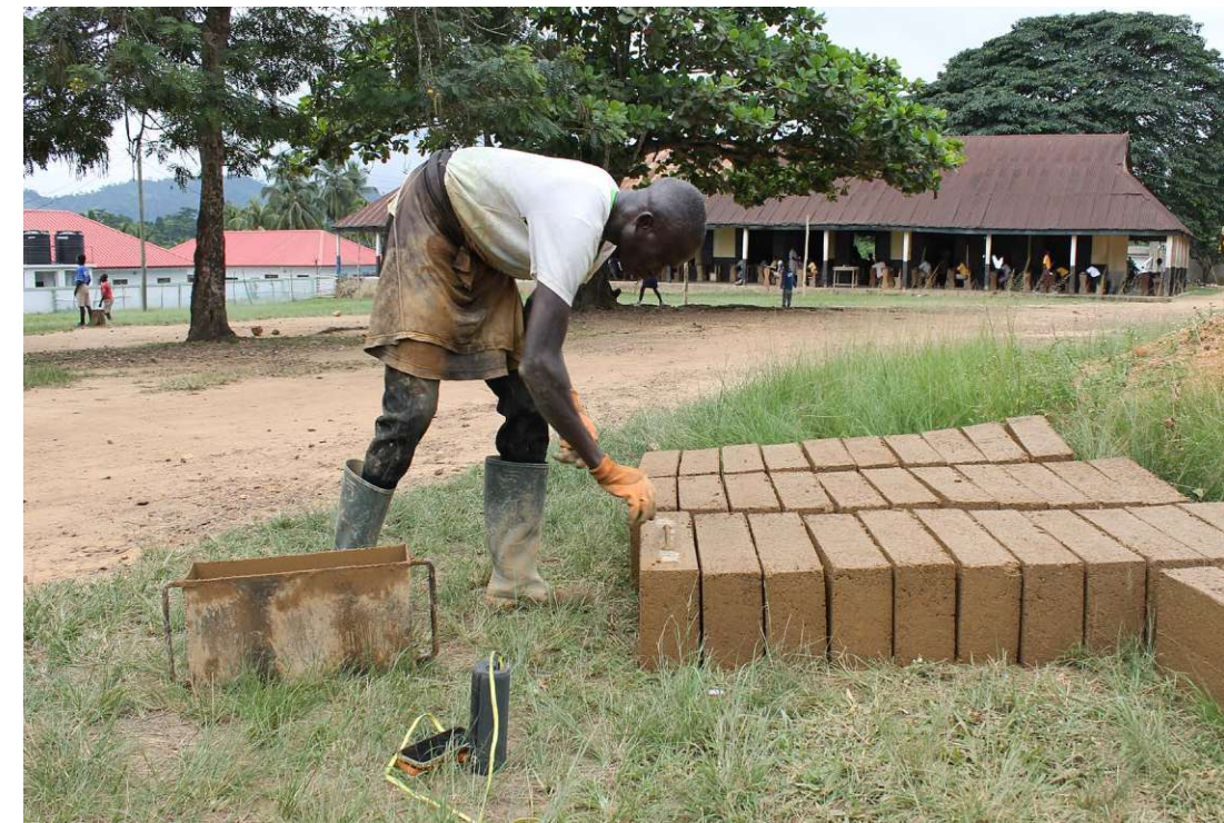
Fig.47: In the end, the bricks get placed in the sun to dry.
