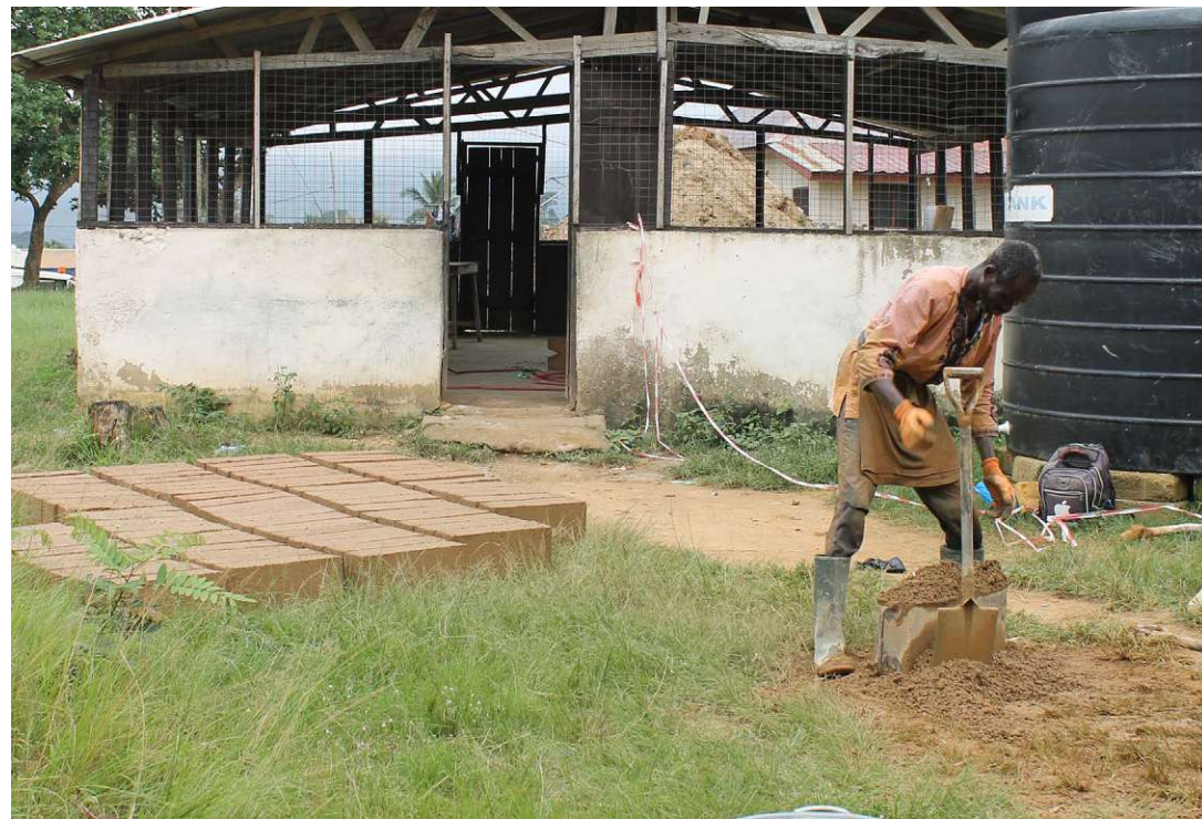
Fig.45: The mixture gets filled into a brick mould & compacted.
