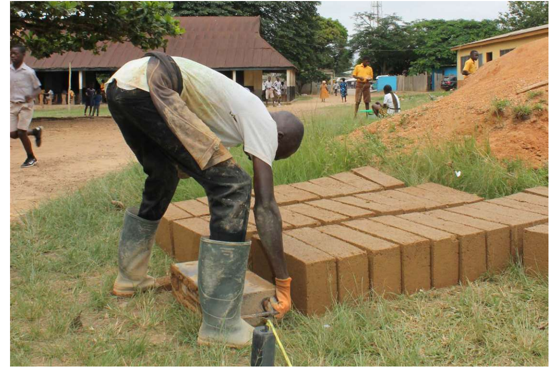
Fig.46: After that, the brick mould gets turned over to remove the brick from it.
