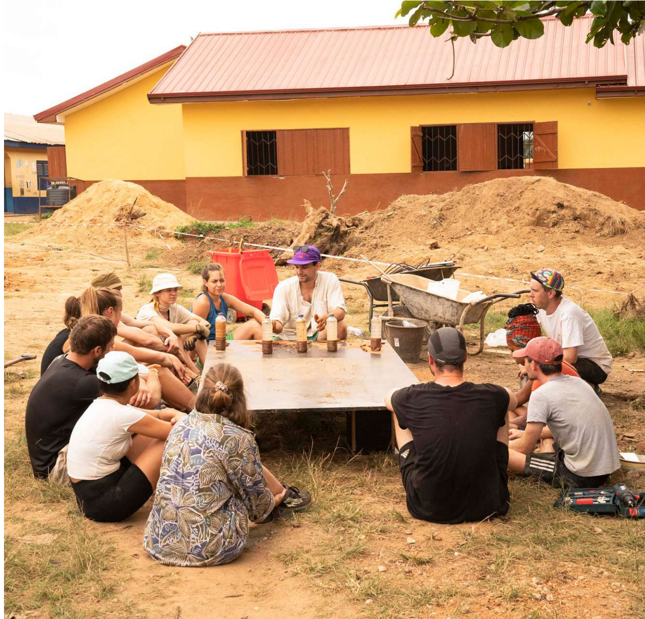
Fig.156: Lorenz Kastner demonstrating the sedimentation test to the volunteers
