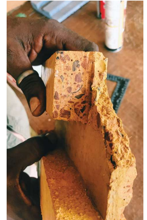
Fig.23: Sun-dried earth tiles with crushed palm nuts
