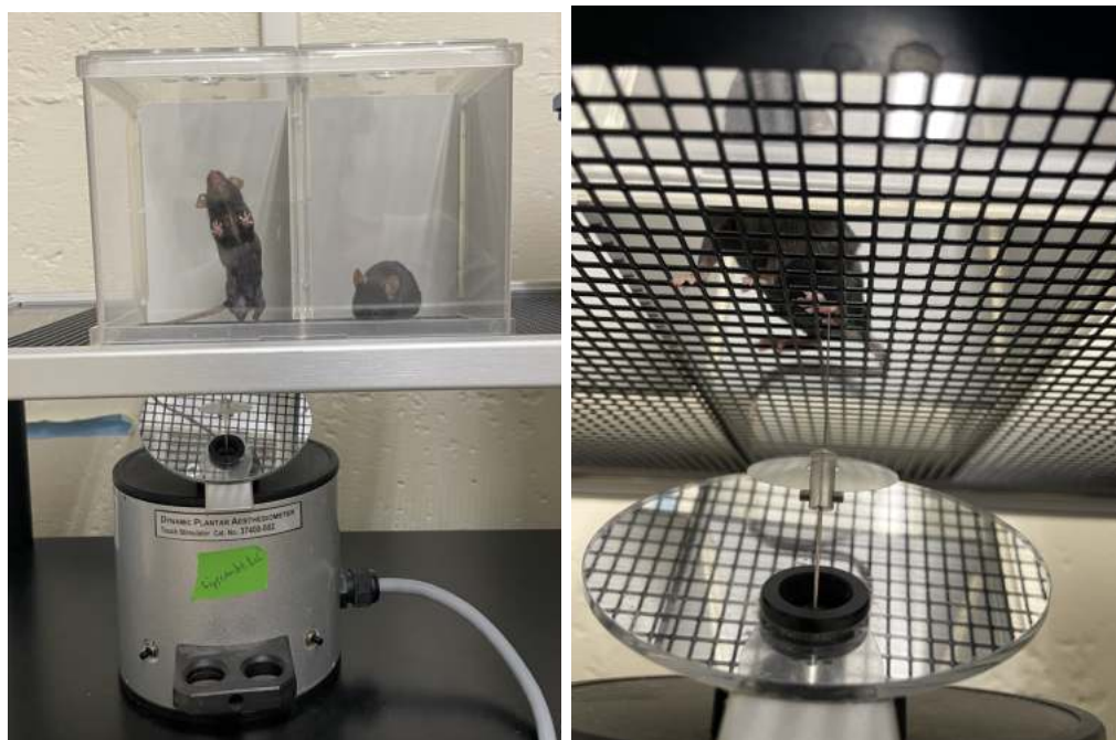
(a) Ugo Basile® Dynamic Plantar Aesthe- (b) force application on hind paw by steel siometer 37450 rod
