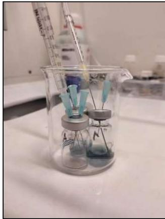
Figure 32: Purging of photocatalysis samples with argon.
