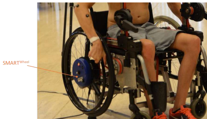
Figure 6: SMART Wheel installed on the right side of the test rig during experiments with paraplegic subjects
