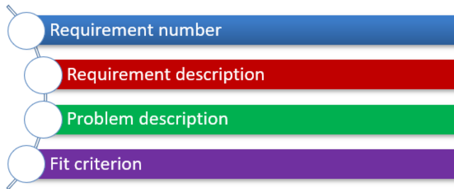
Figure 11: Functional Requirement Structure [47]
