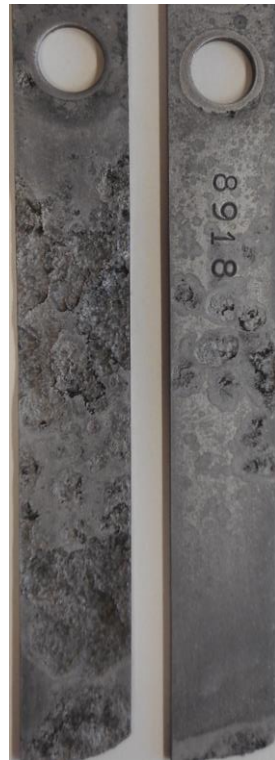
Figure 19: Corrosion coupon with HPAM (P1) at wellhead 1 and localized corrosion attack.
