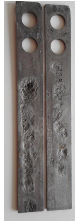
Figure 20: Corrosion coupon with HPAM (P1) at wellhead 2 and localized corrosion attack
