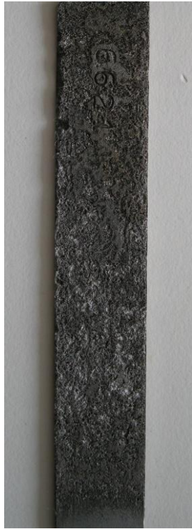
Figure 18: Corrosion coupon without HPAM (P1) and uniform corrosion attack at low corrosion rates.
