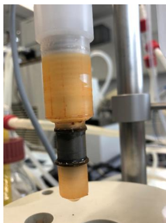
Figure 39: OMV-N1, Test A, corrosion layer on specimen after 24h EIS.
