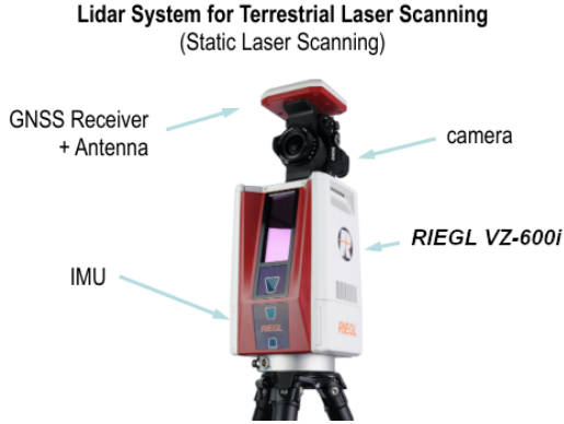
Figure 1: RIEGL VZ-600i terrestrial laser scanner with onboard IMU and RTK-GNSS.
