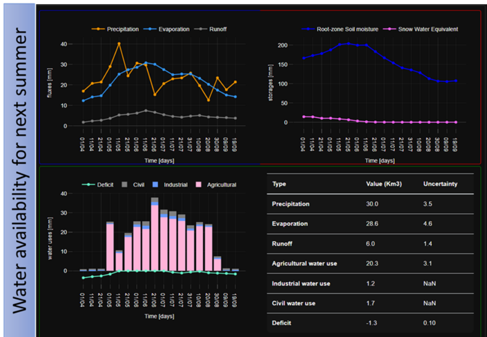
Figure 25: What-if scenario for the next summer period based on the seasonal forecast of precipitation and air temperature and the initial state of soil moisture and snow water equivalent.
