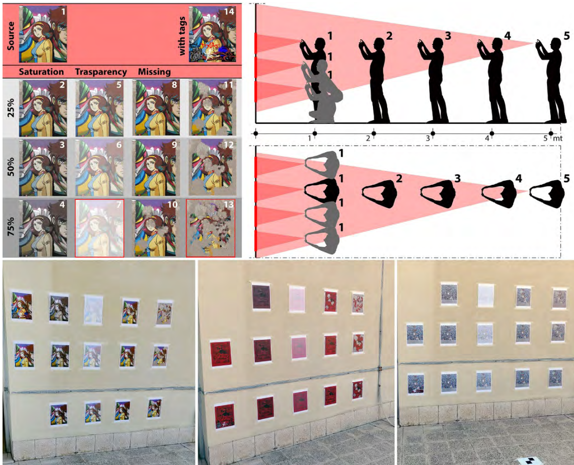
Figure 6. Above is the diagram of the outdoor experiment. The image set refers to the work “Jeeg Robot,” but we replicate the experimentation on the other two works with three different smartphones. Bottom the three different scenarios of the experimentation on the three works.
