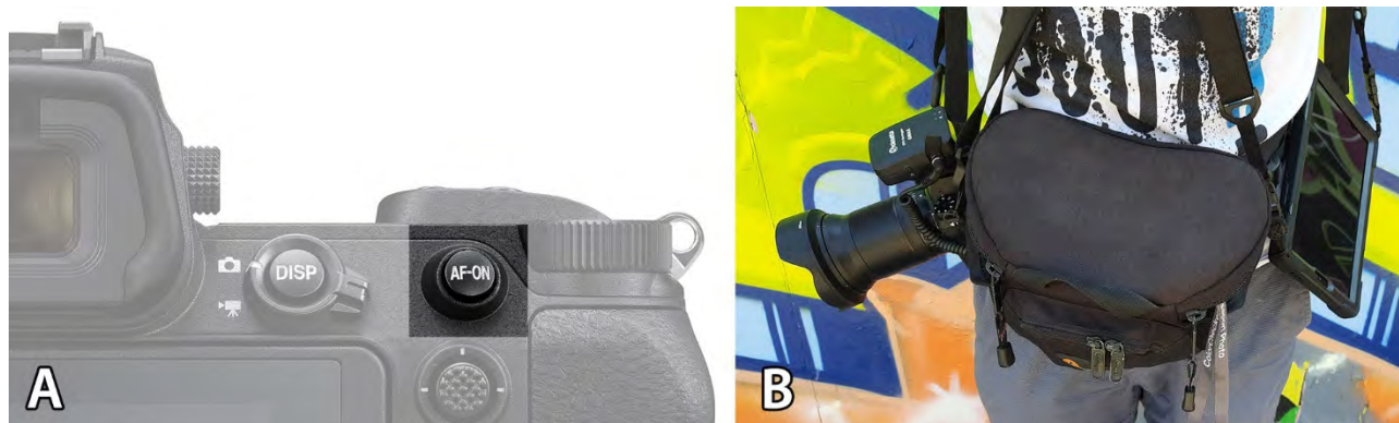
Figure 9. (A) The AF-ON button on the back of the Nikon Z7II. (B) shows one possible combination of carrying all hardware during a follow-up photography tour: the camera and tablet (in a protective case) feature a camera strap worn diagonally over the body, while a pouch carried in front holds the colour reference target and the spectrometer. The pouch protects these sensitive instruments without compromising easy access.
