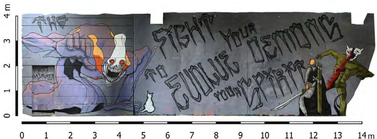
Figure 3. Example of a graffiti orthophotomap with a uniform scale. Within this orthophoto, we can measure distances, angles and areas. The perimeter of this graffiti is 36.82 m, and its area equals 51.2 m 2 , making it one of the largest graffiti along the Donaukanal as of November 2021
