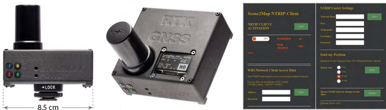
Figure 12. The new RTK-enabled GNSS logging device (left and middle) with the interface controlling its settings (right).
