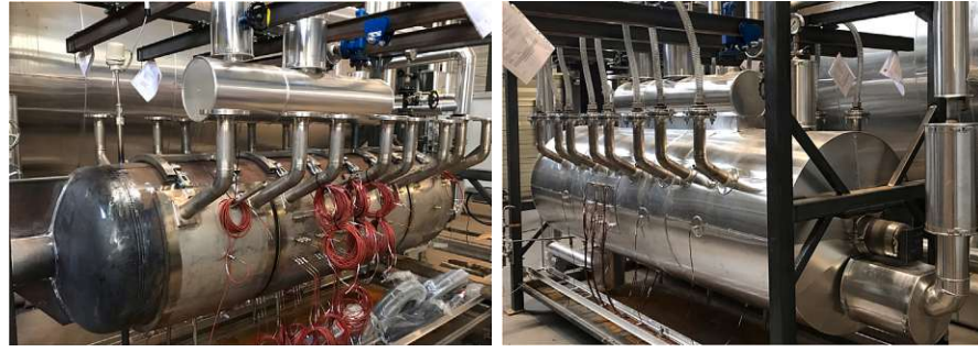
(a) Lab-scale RSS device with LHTES container modules attached to the pressure vessel's surface. The modules are instrumented with PT100 temperature sensors. (b) Final experimental setup of the hybrid storage prototype, including heat insulation.
